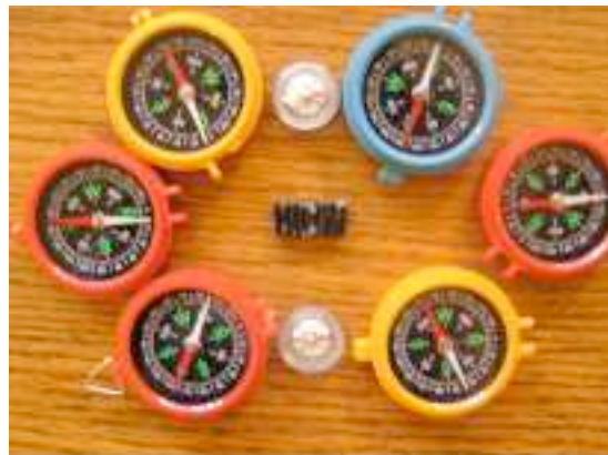
You can see how the compass needles are following the field lines.
